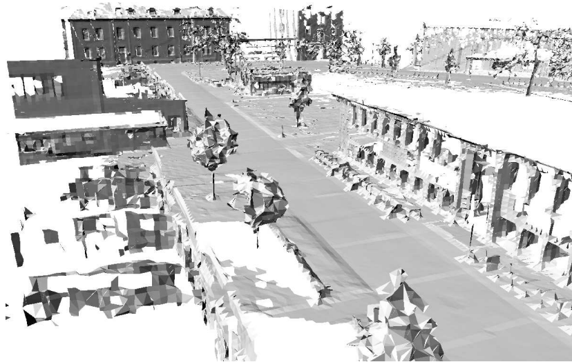
Figure 9: Triangulated mesh representation of the outer loop including data points from 77 laser scans. Extension 2 shows a virtual walk through this model on the trajectory taken by the robot. Figure 10 depicts the elevation map of the same scene.
