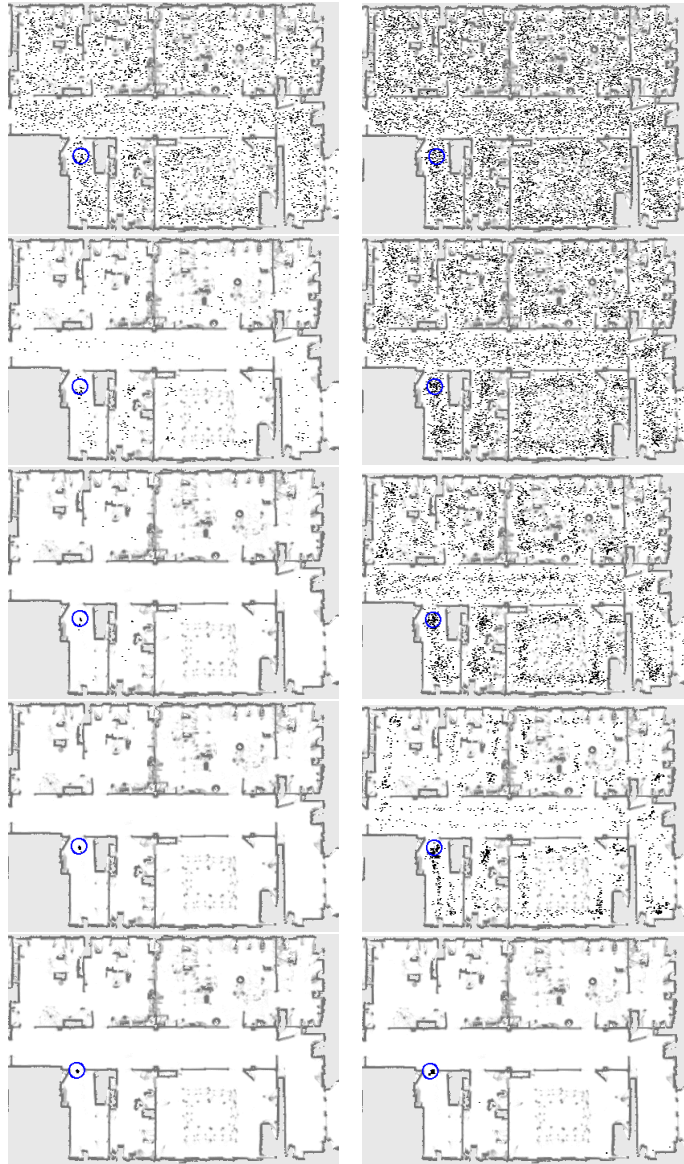
Fig. 4. Distribution of 10,000 particles after 1, 2, 3, 5, and 11 integrations of measurements with our dynamic sensor model (left column) and with the best static sensor model (right column).
