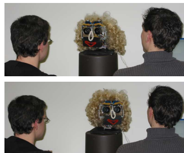
Fig. 1. A conversation of our robot Alpha with two people. As can be seen, the robot shifts its attention from one person to the other to include both into the conversation.
