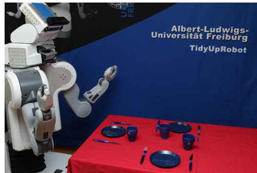
Fig. 1. A scene typically contains several observable objects and the task is to infer the latent meta-objects where a meta-object is considered to be a constellation of observable objects. At a breakfast table, for example, the meta-objects might be the covers that consist of the observable objects plate, knife, fork, and cup.
