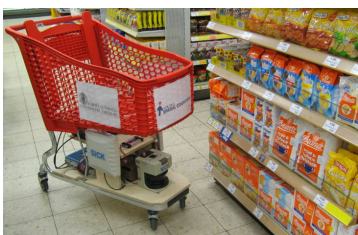
Fig. 6: We equipped a shopping cart with an RFID reader and a laser range scanner and deployed about 350 passive UHF tags in a supermarket.
